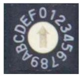
Ignition rotary switch location on MezIO™ board
