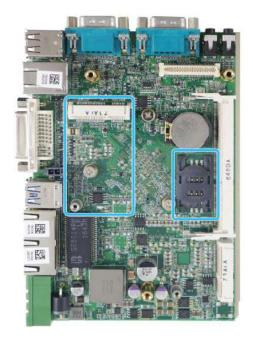
mini-PCle/ SIM slot on MezIO™ module
