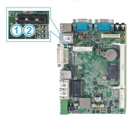
3. When the latched switch is closed, the DC power is in break-off status and system is turned off. When the latched switch is opened, the DC power is in feed-in status and with the correct setting of "Power On after Power Failure" BIOS option, the system is turned on.
