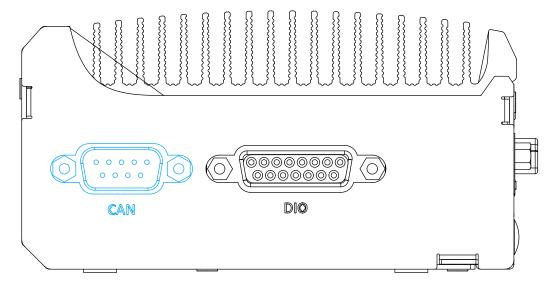
CAN bus is a robust industrial bus with a pair of differential signals and is commonly used in various industrial and in-vehicles applications. The system is equipped with a CAN bus DB9 port that is compatible with both industrial and in-vehicle applications. The CAN bus port supports CAN2.0A and CAN2.0B up to 1Mbps.
