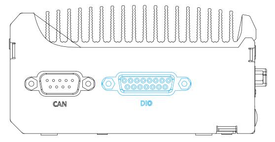
The system provides 4x isolated digital input channels and 4x isolated digital output channels. The DIO functions support polling mode I/O access and DI change-of-state interrupt. Please refer to <a href="Watchdog Timer & Isolated DIO">Watchdog Timer & Isolated DIO</a> for information on wiring and programming the isolated DIO channels.
