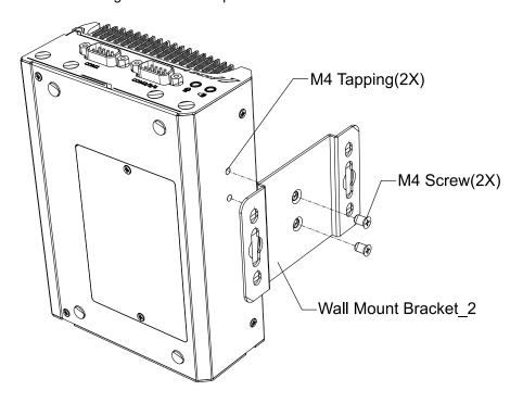
2. Dimension illustration of the install vertical wall mount bracket for you reference.
