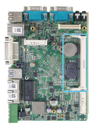
The system has an internal SO-DIMM slot supporting DDR3L-1866 memory module up to 8GB in capacity. The L in DDR3"L"-1866 denotes Low Voltage (1.35V) type SO-DIMM memory modules.
