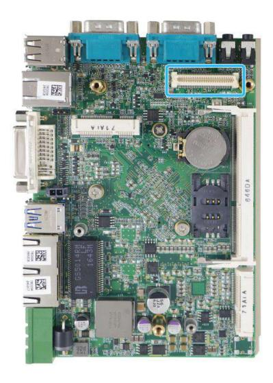
MezIO<sup>TM</sup> is an innovative interface designed for integrating application-oriented I/O functions into an embedded system. It offers computer signals, power rails and control signals via a high-speed connector. MezIO<sup>TM</sup> is also mechanically reliable benefited from its 3-point mounted mezzanine structure. A MezIO<sup>TM</sup> module can leverage these signals to implement comprehensive I/O functions.
