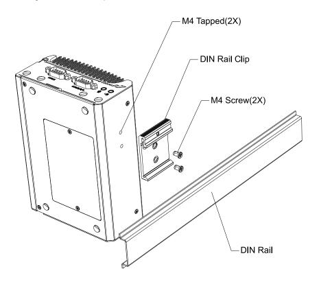
To install the DIN rail clip onto the DIN rail, you must come over the top of the DIN rail, tilting, overlap the top clip edge of the DIN rail clip onto the DIN rail first, and then firmly press the bottom-front of the enclosure to clip the bottom edge of the mount plate.
