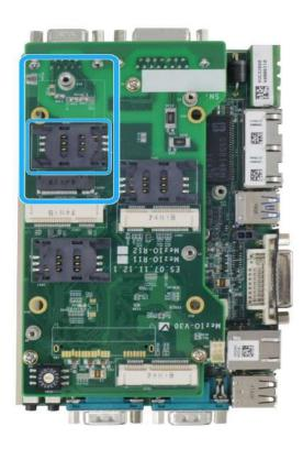
3. To insert a SIM card, push and flip the slide-and-clamp slot towards the center of the MezIO<sup>TM</sup> module.
