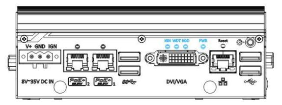
There are four LED indicators on the front panel: PWR, HDD, WDT and IGN. The descriptions of these four LEDs are listed in the following table.
