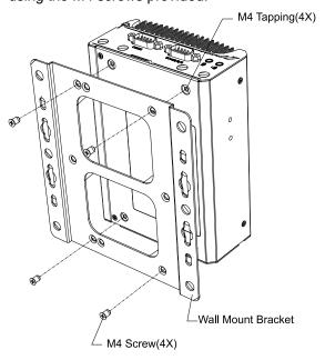
2. Dimension illustration of the install wall horizontal mount bracket for you reference.
