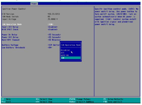
If you wish to set the power on delay time from when you start-up the vehicle, highlight and select "Power On Delay", select the timing according to your needs and press Enter.
