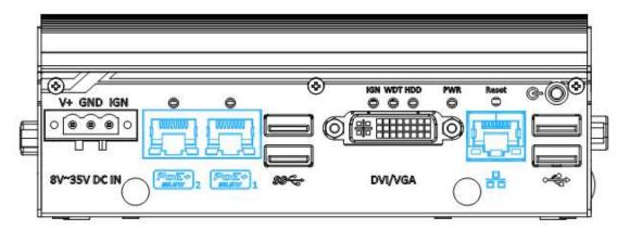
The system offers three Gigabit Ethernet ports using Intel® I210 GbE controller. From top to bottom, they are port #3, #1 and #2. When plugged in and connected via the Ethernet cable, the LEDs on the RJ45 connector indicate connection status and speed.
