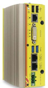
External connection wise, POC-351VTC has three Gigabit Ethernet ports (two are 802.3at Gigabit PoE+
