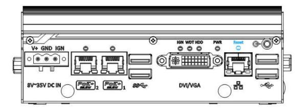
The reset button is used to manually reset the system in case of system halt or malfunction. To avoid unexpected reset, the button is purposely placed behind the panel. To reset, please use a pin-like object (eg. tip of a pen) to access the reset button.
