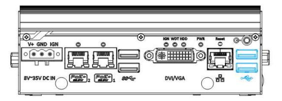
The USB2.0 ports are implemented via native xHCI (eXtensible Host Controller Interface) controller in Atom E3950 is backward compatible with USB 1.1 and USB 1.0 devices. Legacy USB support is also provided so you can use USB keyboard/mouse in DOS environment.
