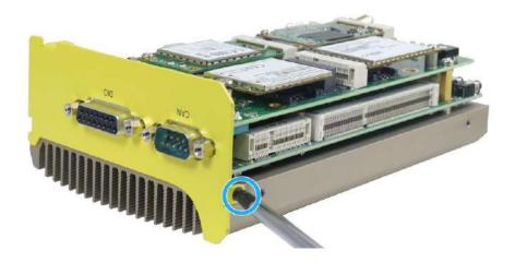
2. Install the front panel and secure it with two (2) screws indicated in the illustration below.
