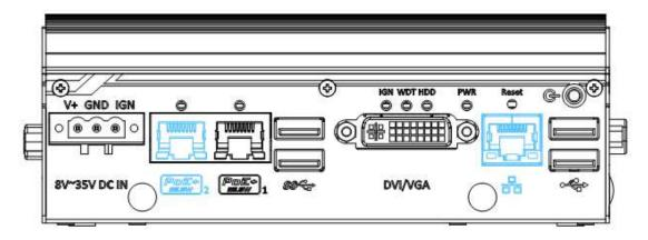
The Power over Ethernet (PoE) port supply power and data on a standard CAT-5/CAT-6 Ethernet cable. Acting as a PSE (Power Sourcing Equipment), compliant with IEEE 802.3at, each port delivers up to 25W to a Powered Device (PD). PoE automatically detects and determine if the connected device is PoE PD or not before supplying power, making it compatible with standard Ethernet devices as well.
