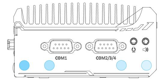
The system offers four SMA antenna openings reserved for SMA antenna installations. Users can take advantage of these two openings when installing mini-PCle module for wireless communication reception such as 3G, 4G, GPS or WiFi.
