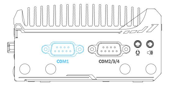
Implemented using industrial-grade ITE8786 Super IO chip (-40 to 85°C) and provide up to 921600 bps baud rate, COM1 is a software-configurable RS-232/422/485 port via 9-pin D-Sub male connector. The operation mode, slew rate and termination of COM1 can be set in BIOS setup utility. The following table describes the pin definition of COM ports.
