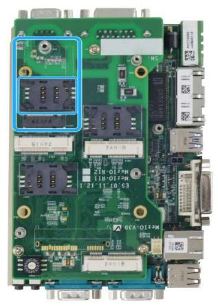
The M.2 socket (2242/ 3042) accepts USB signal only and is coupled with SIM card support. By installing a 3G or 4G M.2 module with a SIM card, you can access the internet via your service provider's 3G/4G network.
