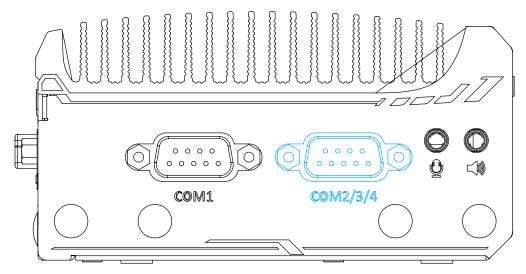
Implemented using industrial-grade ITE8786 Super IO chip (-40 to 85°C) and provide up to 921600 bps baud rate, the second D-Sub male connector (COM2/ 3/ 4) can be configured in BIOS as single RS-422/ 485 port (COM2) or three 3-wire RS-232 ports (COM2/COM3/COM4). Please refer to COM2/3/4 Port Configuration for configuring operation mode. An optional 1-to-3 Y-cable is available to connect three RS-232 devices.
