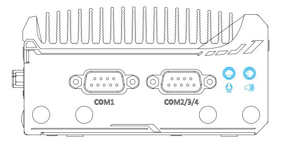
The system provides audio function using Intel® High Definition Audio in Atom E3950 SoC and Realtek ALC262 codec. There are two audio jacks on the top panel. The port is used for microphone input, and port is used for speaker output. To utilize the audio function in Windows, you need to install corresponding drivers for both Intel® HD audio and Realtek ALC262 codec. Please refer to the section, <a href="Driver">Driver</a> Installation.
