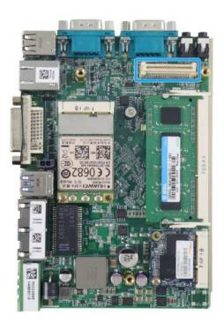
The stand-off hex bolts can be located on the mainboard. Place the MezIO<sup>™</sup> module on top of the mainboard, match the three hex bolts and the MezIO<sup>™</sup> connector should meet.
